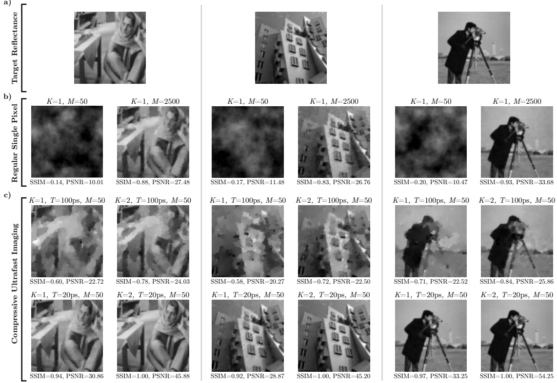
Figure 3-12: FemtoPixel simulation results. a) The target image. b) Result with a regular single pixel camera with M = 50 and M = 2500 patterns. c) Results with compressive ultrafast sensing with M = 50 for four design points with time resolution of T = 100 ps and T = 20 ps, and K = 1 and K = 2 . All reconstructions are evaluated with SSIM and PSNR. The results demonstrate the strong dependency on time resolution. Recovery with K = 2 and T = 20 ps shows perfect reconstruction on all targets based on SSIM. All measurements were added with white Gaussian noise such that the measurement SNR is 60 dB.
